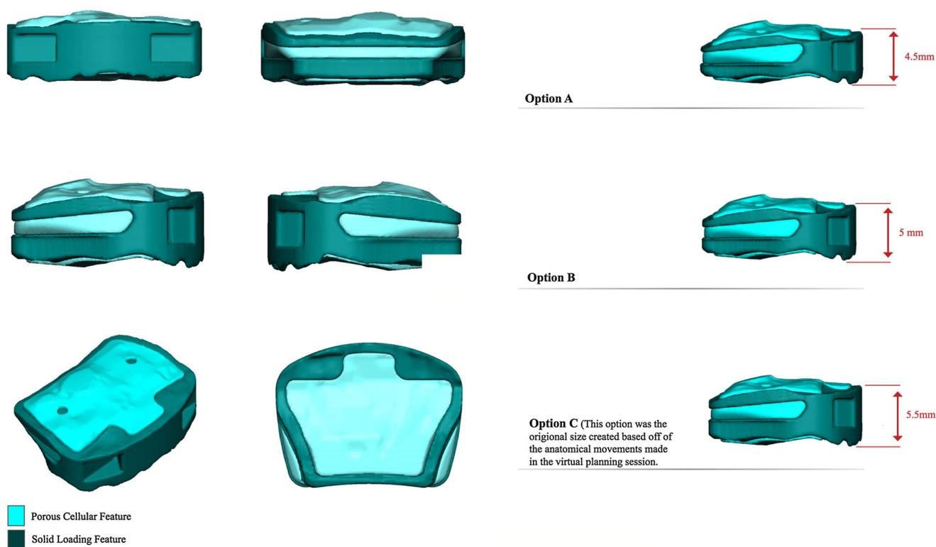
**Fig. 5** Finished design of the individual implant with three different heights in 0.5 mm steps
