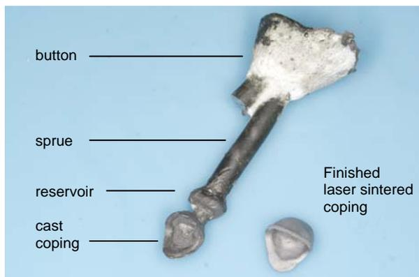
**A cast coping (left) and a finished laser sintered coping (right)**
